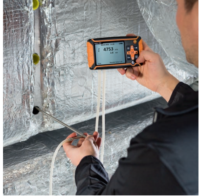
Removable instrument allows Pitot tube measurements in ducts (Pitot tube available separately)
