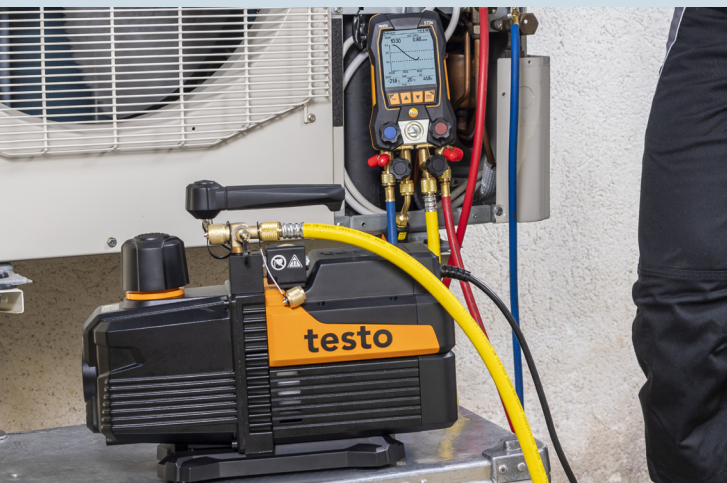
Non-return valve to prevent vacuum loss in the event of a power interruption
