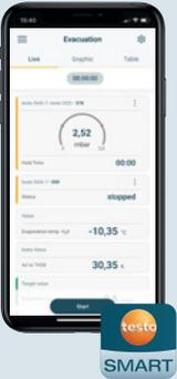
The testo Smart App guides you quickly and easily through measurements on refrigeration, air conditioning and heating systems.
